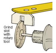
To do this, simply cut a small slot on the hook with a rotary tool (or hack saw), see the drawing above right.
