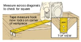
The slot slips over the point of the corner of the project, see the drawing and detail at left. The slot holds the tape in place for those large projects where an extra set of hands would be a big help. And it doesn't effect the tape measure's accuracy when I use it for other projects.
